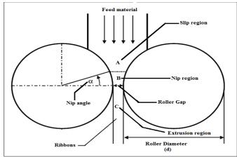
Figure No: 1 Process of roller compaction
