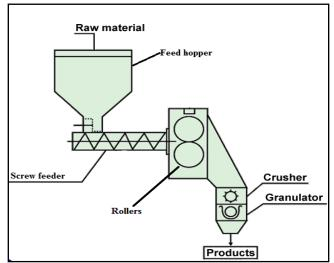
Figure No 3: General diagram of roller compactor
