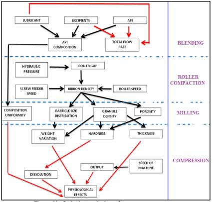
Figure No 2: An interrelation of process parameters
