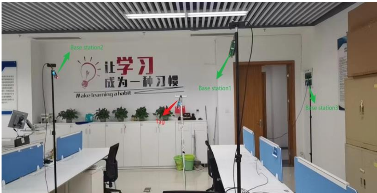
Figure 9. Physical construction of the trilateral positioning system. The system consists of three base stations and a label, and the distance between the three base stations can form three circles, and the intersection of the three circles is solved to be the coordinates of the label.
