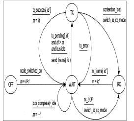
Figure 5 Protocol automaton for the MUST protocol
