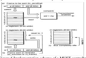
Figure 6 Implementation scheme of a MUST controller with eight priority classes
