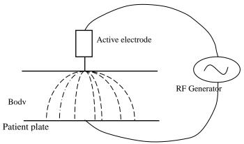
Fig.3 Basic principle behind the electrosurgical machine.
