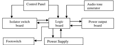
Fig.4 Block diagram for surgical diathermy machine.
