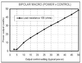
Fig. 7 Graph of Power vs. Control for Bipolar diathermy
