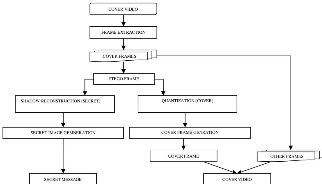
Fig.3 Block Diagram (Decryption System)
