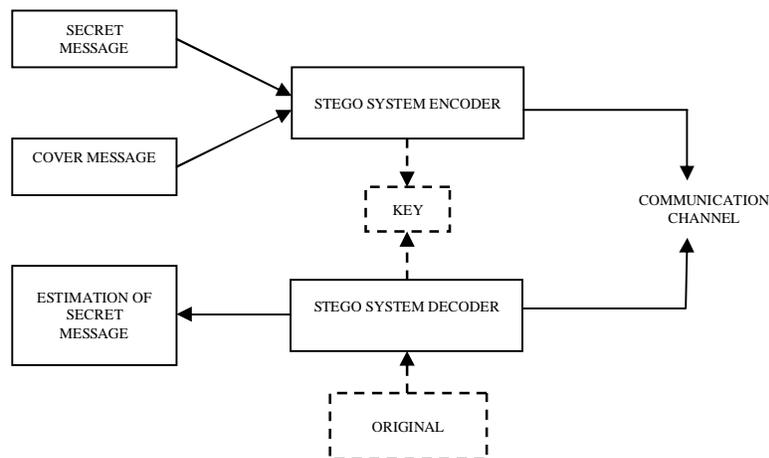
Fig.1 A Basic Steganographic Architecture
