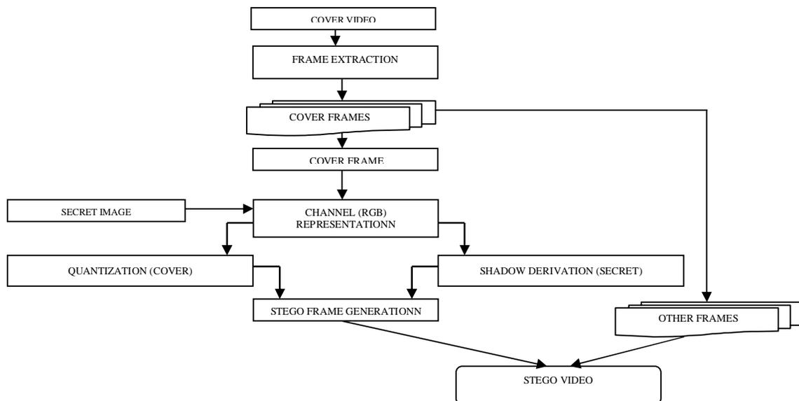
Fig.2 Block Diagram (Encryption System)
