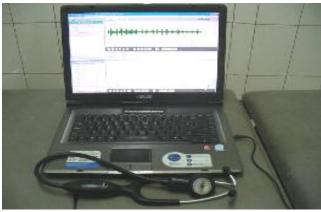
Fig. 2 Jabes electronics stethoscope with laptop based phonocardiogram
