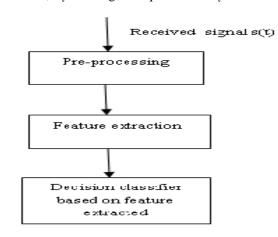
Fig. 1 Modulation Clsssification Model
