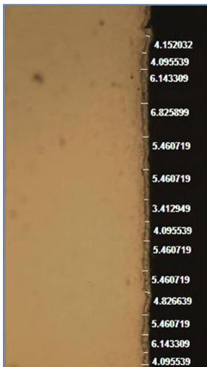
**Figure 2:** Analysis of optical microscopy of cross-DLC coating profile showing the measurement positions.
