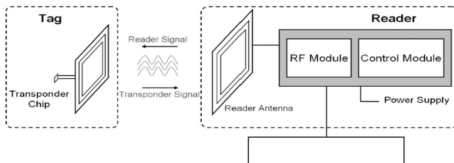
Figure1: Components of an RFID system
