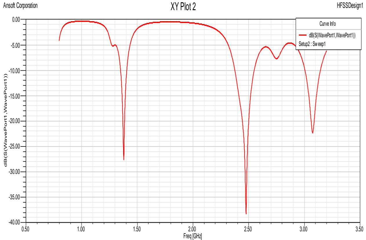
Fig.2 Return Loss (S<sub>11</sub>) parameter of the antenna
