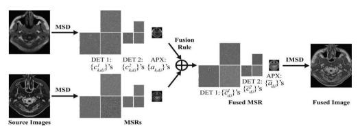
Figure 3.General procedure of MSD-based image fusion in a 2-D case
