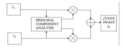
Figure 1.Information flow diagram in image fusion scheme employing PCA
