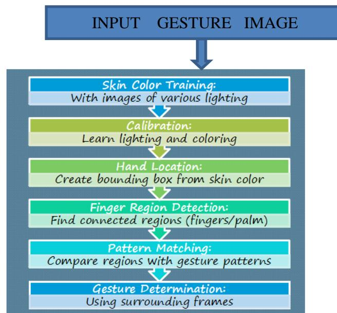
Figure 2 architecture diagram
