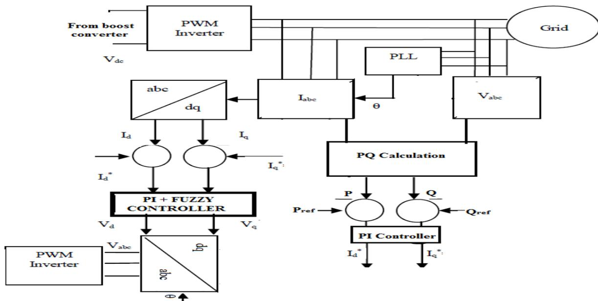
Fig. 5: Control scheme for DC – AC Converter
