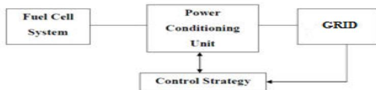
Fig. 6: Block diagram of power conditioning system
