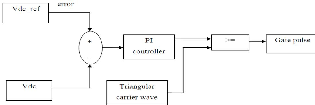
Fig. 4: PI control scheme for DC – DC Boost Converter
