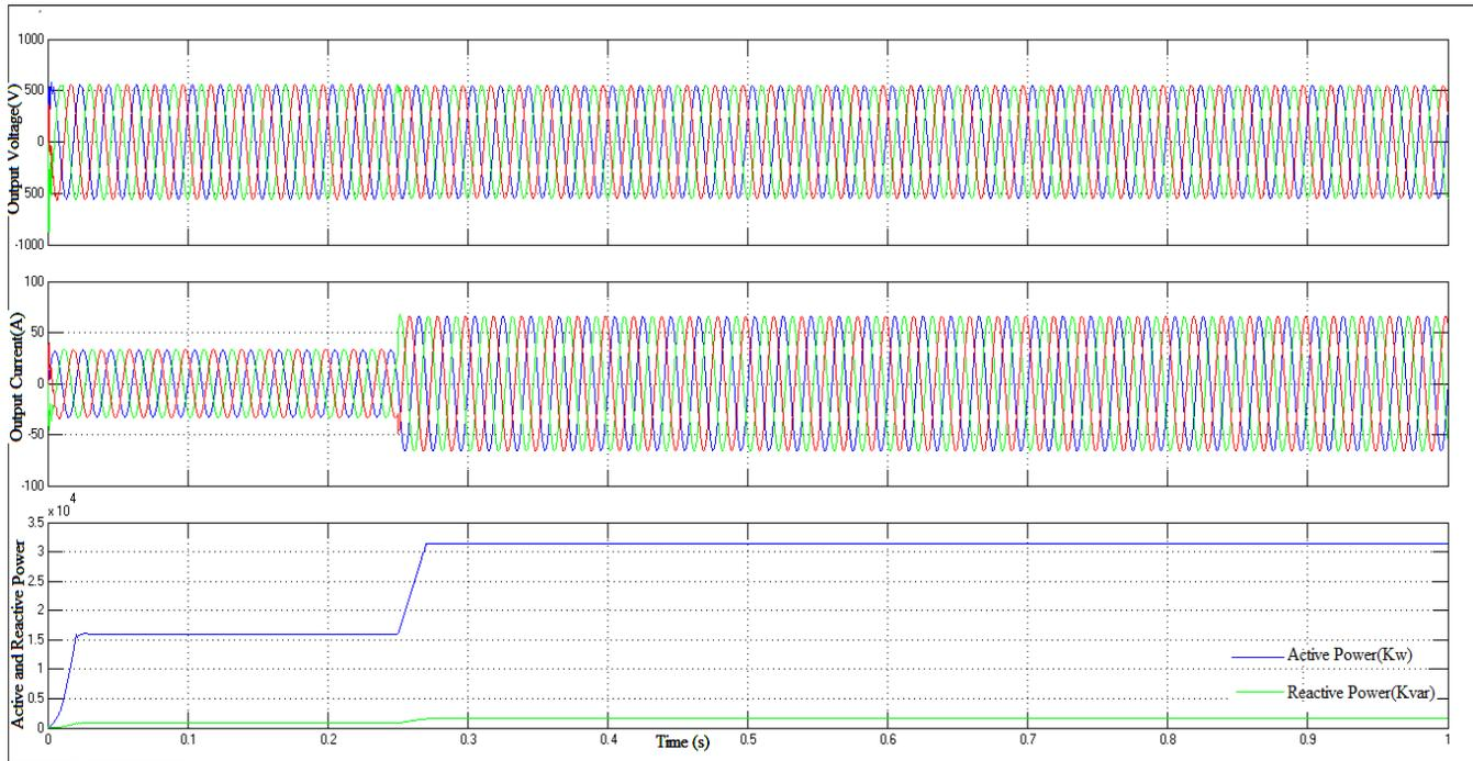
Fig. 9: Simulation results of grid connected inverter
