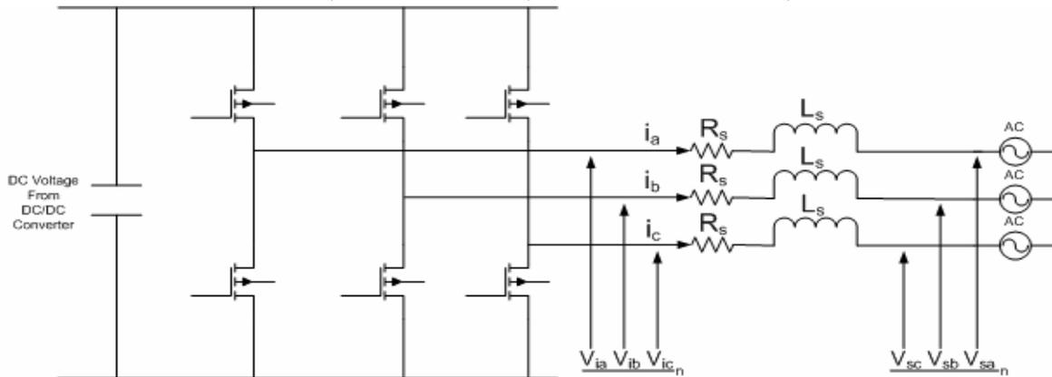
Fig 3: Three-phase dc/ac voltage source inverter
