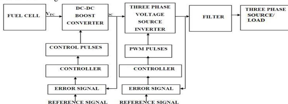
Fig. 1: Block diagram of the FCDG system
