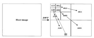
Fig. 1: wavelet decomposition of host image
