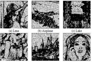
(d) Peppers (e) Sailboat (f) Tiffany Fig. 4. Labels of image blocks with different types (T = 28). The black block, gray block, and white block in Figures 6(a)-(f) correspond to the blocks compressed by VQ, SMVQ, and Arnold coding, respectively.
