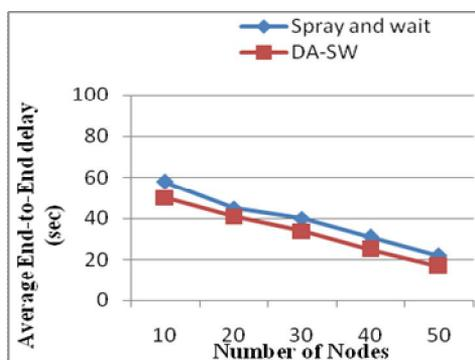
Fig 2: Number of nodes Vs Average End-to-End Delay
