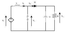
Fig 3.1 Topology of Boost converter
