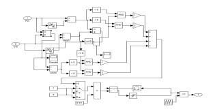
Fig 6.2 Simulation diagram of INC algorithm www.ijareeie.com
