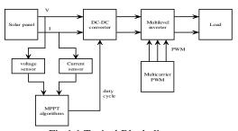
Fig 1.1 Typical Block diagram
