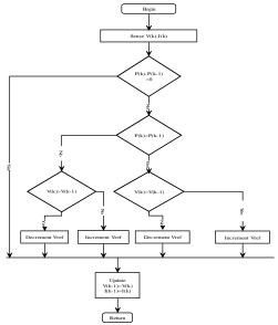
Fig 4.1 Flowchart of P&O algorithm
