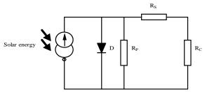
Fig 2.1 Equivalent circuit of ideal PV cell
