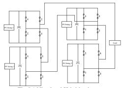
Fig 5.1 Nine level H-bridge inverter
