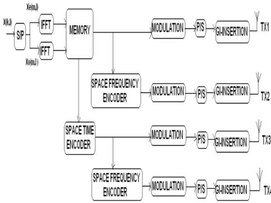
Figure-1:-The diagram of the transmitter end in the four antenna STFC-OFDM scheme.
