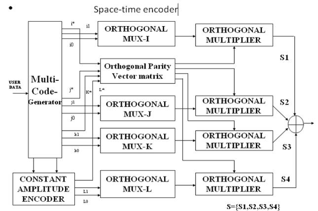
Figure-2 :Block diagram of space time encoder
