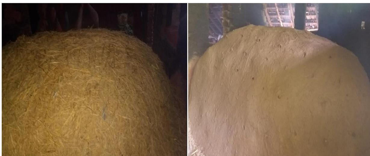
Despite flexibility of fuel can be used, these kilns suffer from low temperature of firing, poor ware strength and extensive breakage.
