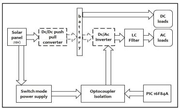
Fig. 2. Micro-inverter system block diagram
