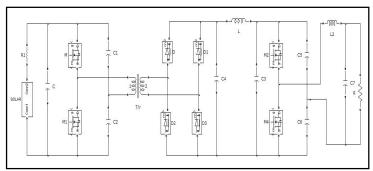
Fig.4. Schematic diagram of DC-AC inverter
