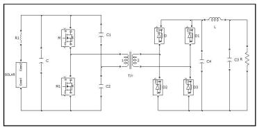
Fig. 3. Push-pull converter circuit diagram
