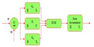
Figure 2 Block Diagram of ADPID
