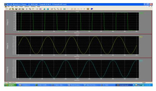
Fig 8: Waveforms of Comparator
