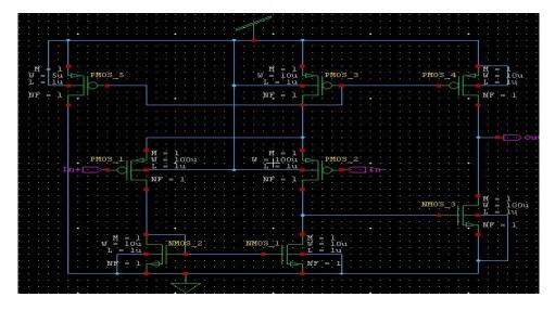
Fig 7: Design of Comparator
