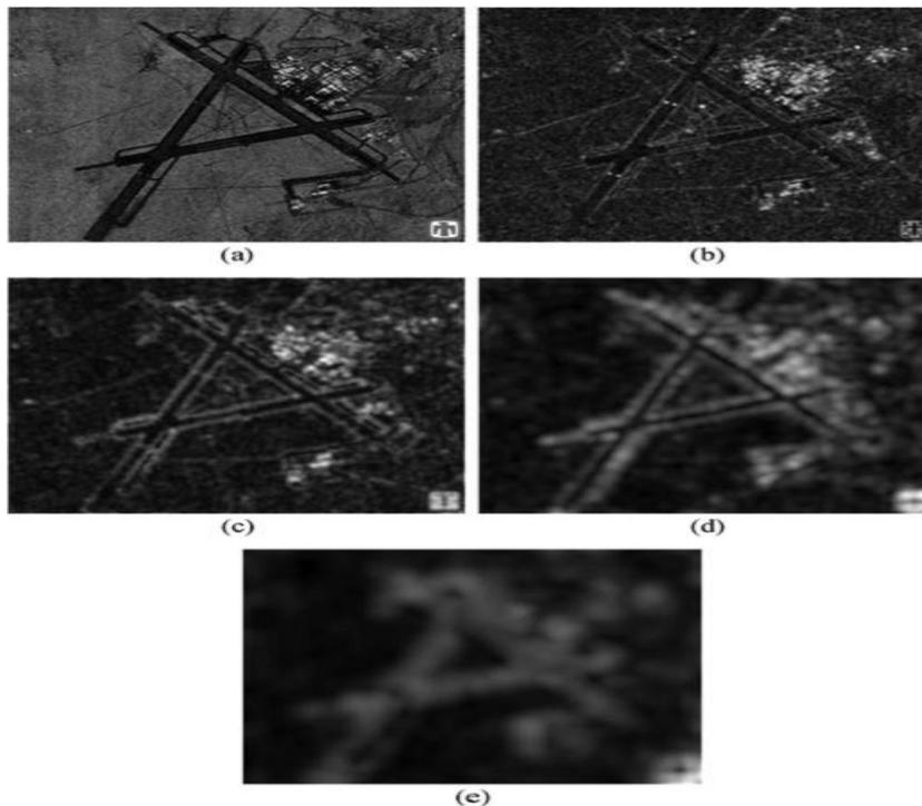
Fig.1. Extracted feature images of a real SAR image for the semantic context.(a) normalized brightness image (b)–(e) isotropic texture images of different scales
