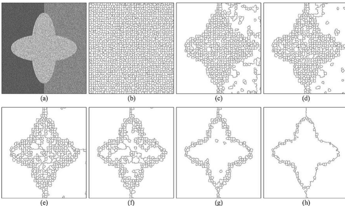
Fig.2. Synthetic SAR image and the intermediate segmentation results of CMS. (a) is the synthetic SAR image. (b) is the super pixels obtained by the preprocessing method. (c)– (h) are the intermediate segmentation results during CMS
