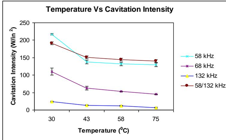
Fig.1 Effect of temperature on cavitation intensity for various ultrasonic frequencies
