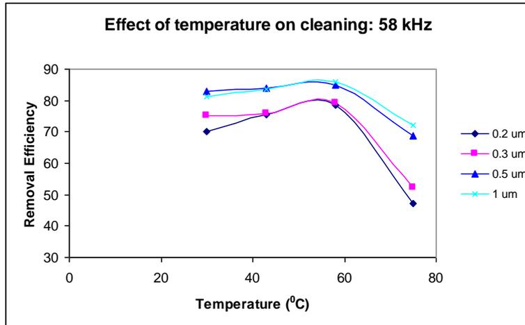
Fig.8 Effect of temperature on particle removal efficiency for 58 kHz
