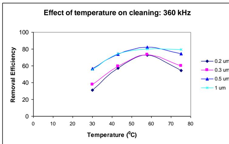
Fig.9 Effect of temperature on particle removal efficiency for 360 kHz
