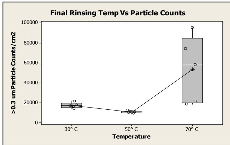
Fig.10 Effect of temperature on particle removal at final rinsing
