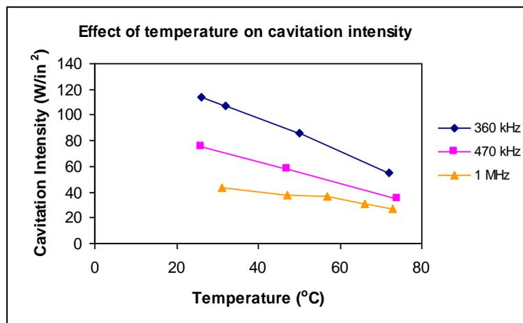
Fig.2 Effect of temperature on cavitation intensity for various megasonic frequencies
