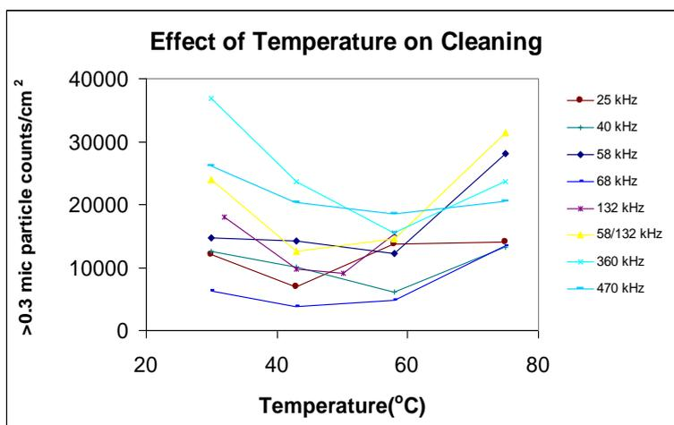
Fig.6 Effect of temperature on cleaning for various frequencies
