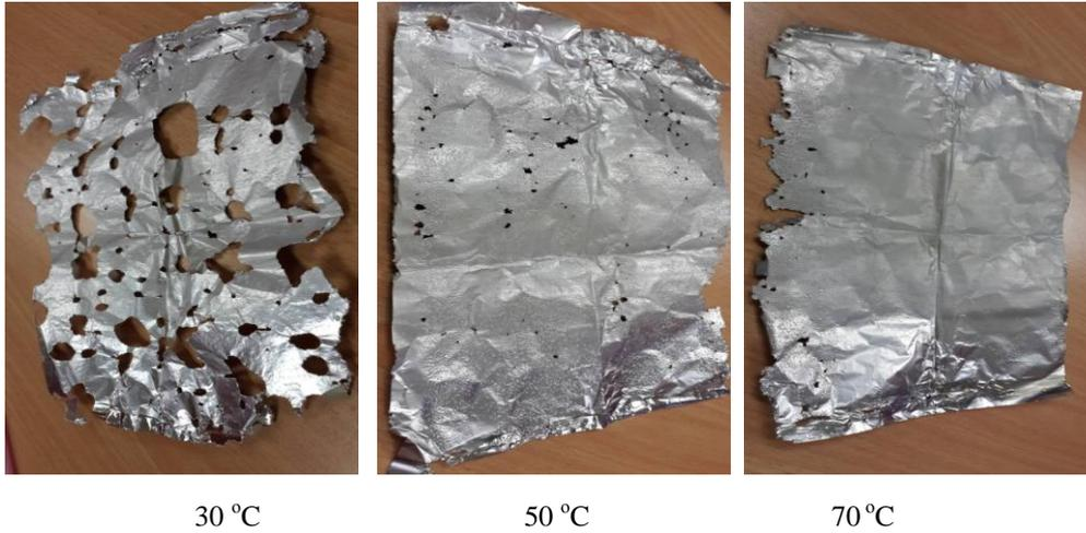
Fig.3 Visualisation of cavitation pattern on aluminium foil for 25 kHz
