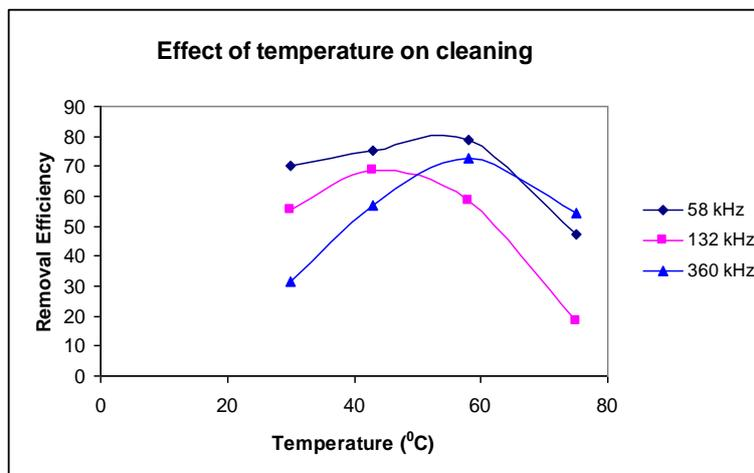
Fig.7 Effect of temperature on cleaning efficiency
