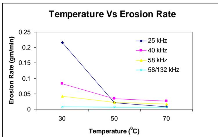
Fig. 4 Effect of temperature on erosion rate
