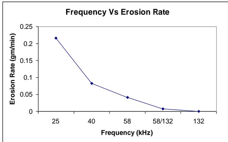
Fig.5 Effect of frequency on erosion rate
