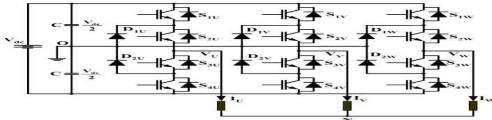
Figure2. Three -level Neutral Point Clamped topology
