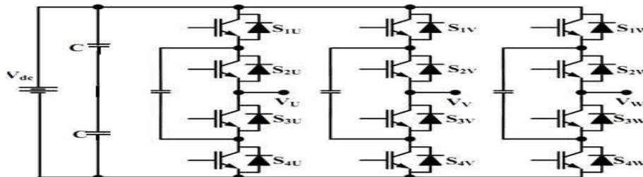
Figure3. Three-level Flying Capacitor topology
