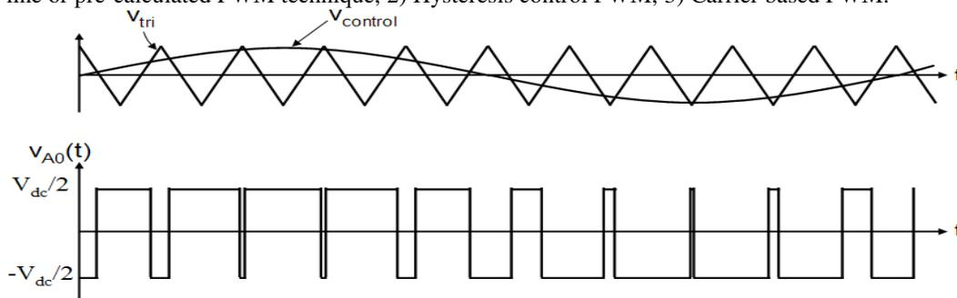
Fig. 4: Pulse-Width Modulation.
