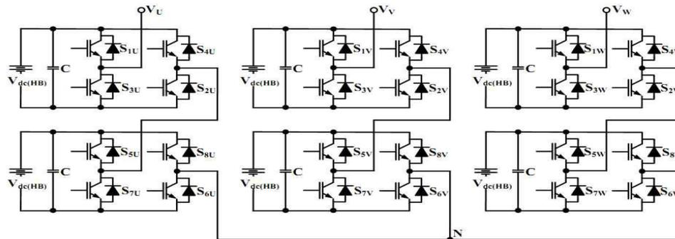
Figure4. Five-level Cascaded H-Bridge Topology
