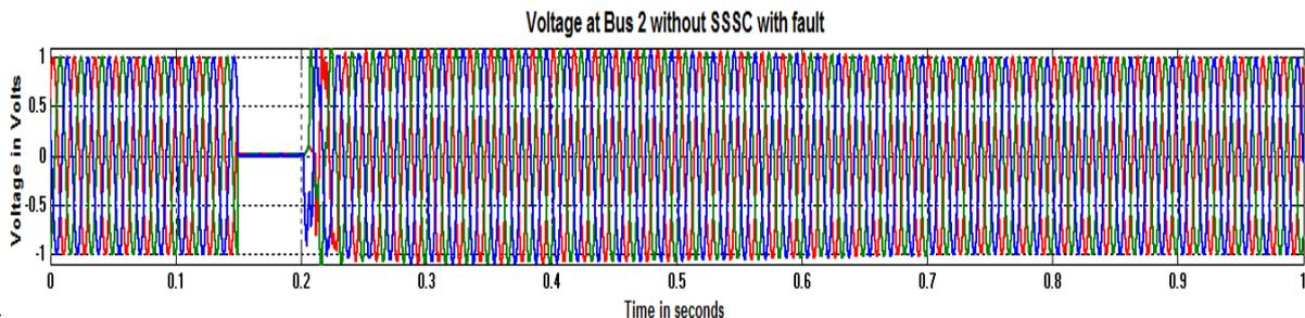
Fig.14: Voltage at bus 2 without SSSC with fault.
