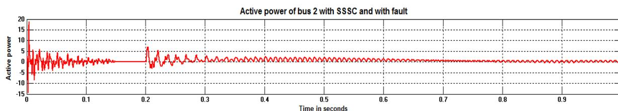
Fig.20: Active power at bus-2 with SSSC and with fault.
