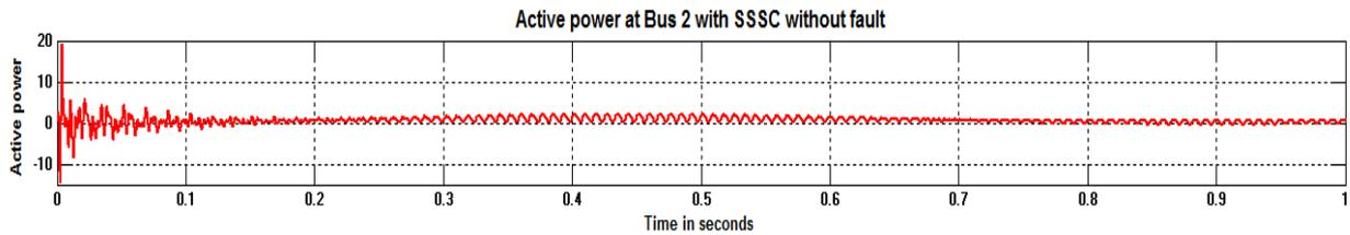
Fig.12: Active power at bus -2 when SSSC is connected.
