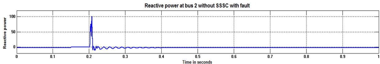
Fig.17: Reactive power at bus 2 without SSSC with fault.
