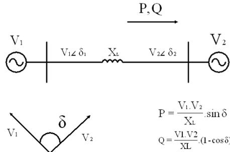
Fig. 1: Simple transmission line.
