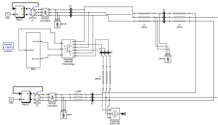
Fig. 4: Two machine power system with SSSC and without fault.
