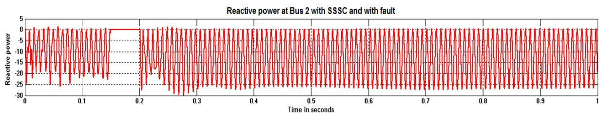
Fig.21: Reactive power at bus-2 with SSSC and with fault.
