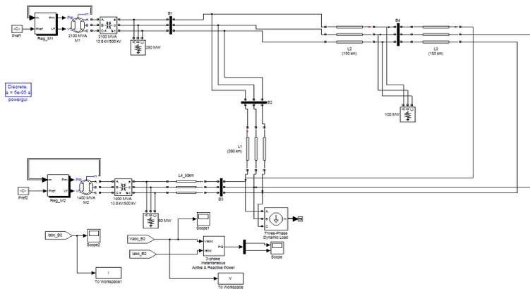
Fig. 3: Two machine power system model in MATLAB (Without SSSC and without fault).
