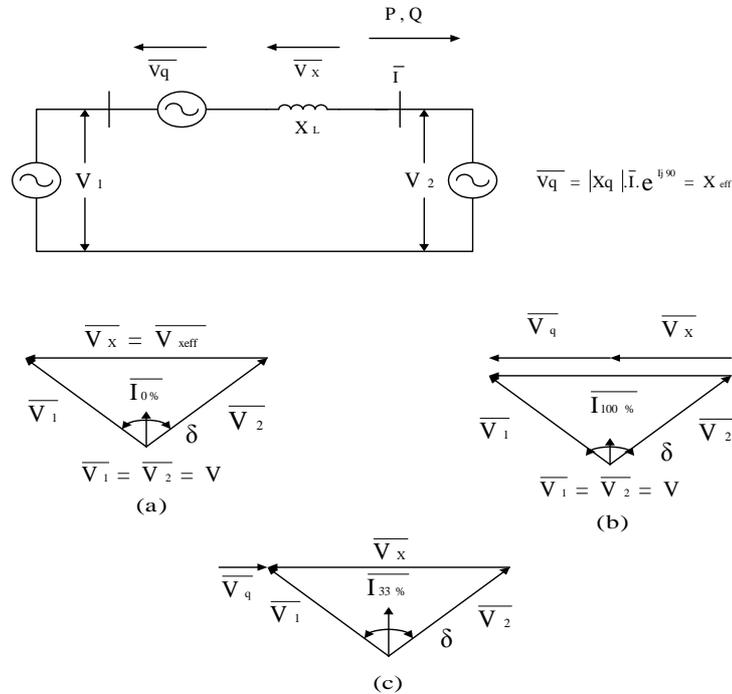
Fig. 2: Transmission line with SSSC connected in series.
