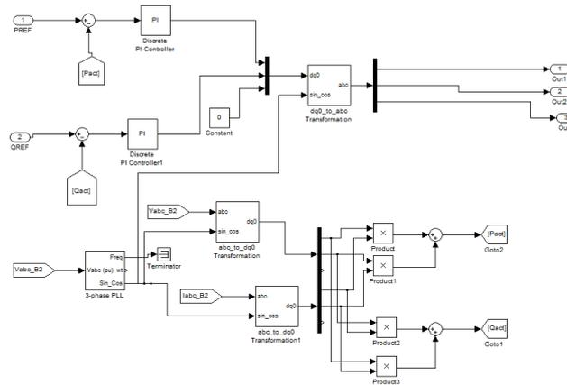
Fig. 5: Control scheme for SSSC.
