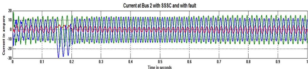
Fig.19: Current at bus-2 with SSSC and with fault.
