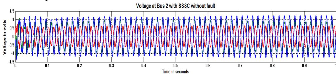
Fig.10: Voltage at bus -2 when SSSC is connected.
