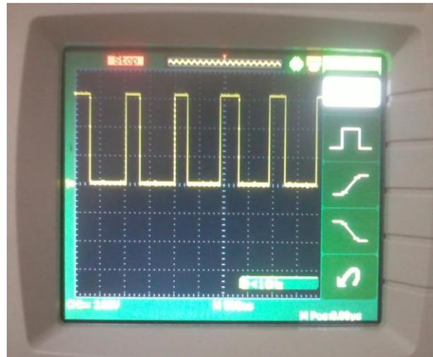
Fig 5.Comparator Output
