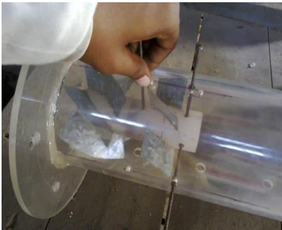
*Fig.4* Rotating swirler with guide vane at 0° inlet & 45° outlet angle.
