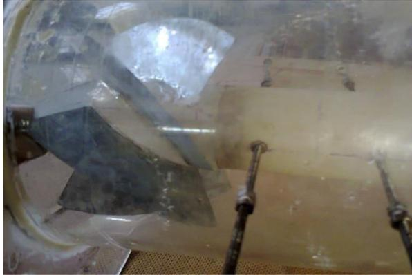
*Fig.2* Rotating swirler without guide vane
