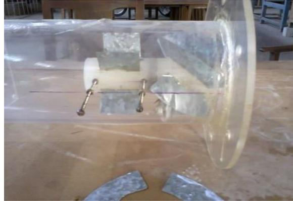
*Fig.3* Rotating swirler with guide vane at 0° inlet and outlet angle
