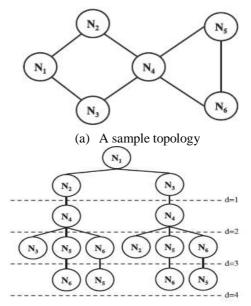
(b) SCF-tree of node N1 Fig 6: SCF-tree based method of replica allocation [2]
