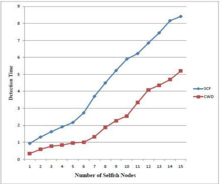
Fig 8: comparison between detection time of SCF-tree base method and watchdog method [11]
