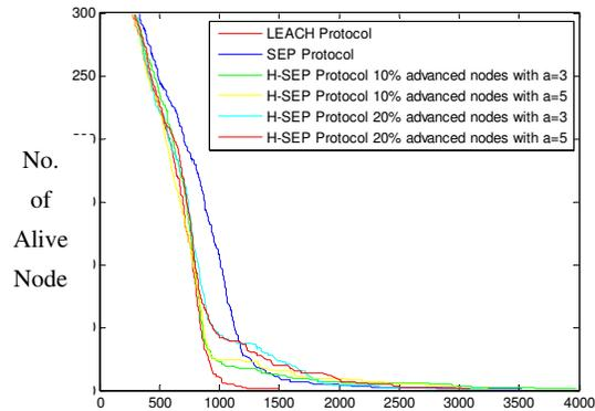
**Figure 5** Number of alive nodes per round in random deployment in square field (LEACH; SEP; H-SEP with  $m=0.1$  and  $a=3$ ; H-SEP with  $m=0.1$  and  $a=5$  for 2-level)
