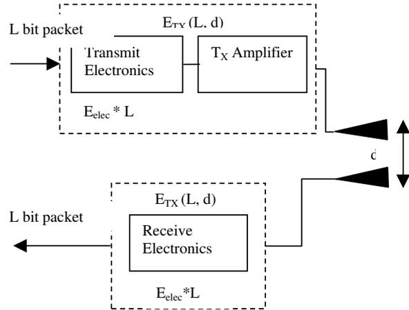
**Figure 1** Radio Dissipation Model
