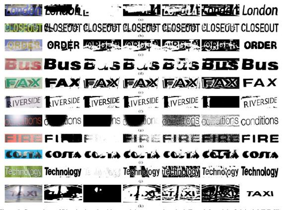
Figure 5. Comparison of Binarization algorithms and the proposed method (From left to right Original, MRF, Kittler, Otsu, Niblack, Sauvola, Proposed); (a)-(d) Text containing reflective background; (e)-(f) Text containing shadowed background; (g)-(j) Text containing specular background; (k) Text containing reflective, shadowed and specular background.
