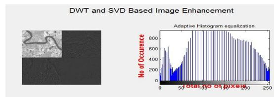
Figure 4 shows Discrete Wavelet Transform of an image. Here the input image is divided into four sub-bands, from that we obtain the wavelet coefficient for each part of the
