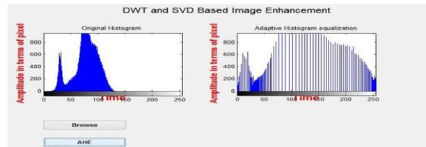
Figure 2 Shows the Adaptive Histogram Equalization[5][7]. By calculating Cumulative distribution function( CDF) ,we get a histogram of an image,.Divides the image into smaller tiles, applies histogram equalization to each tile, then interpolates the results ; here the gray level pixels are distributed evenly this leads to improve the quality of the image.
