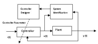
Fig.1 Indirect Adaptive Control using Takagi-Sugeno Fuzzy System
