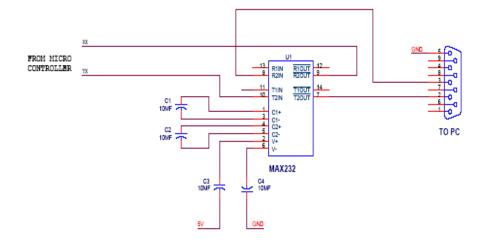
Fig. 5 Connection of MAX 232 with PC
