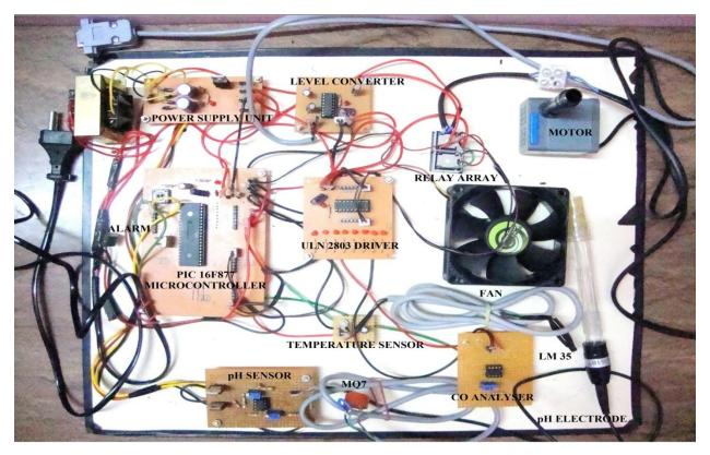
Fig. 7 Hardware setup
