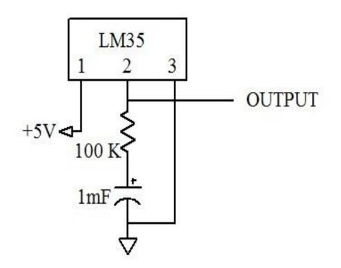
Fig. 3 Temperature analyzer circuit
