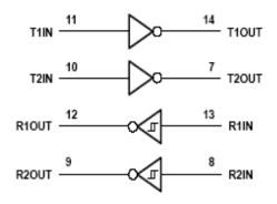
Fig. 6 Transmitter configuration of MAX 232
