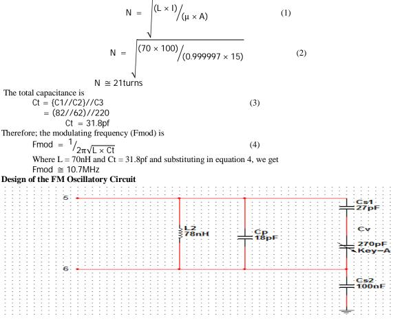
Fig 4: FM Oscillatory Circuit
