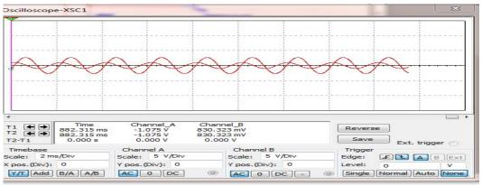
Fig 11: Output Waveform of AM Receiver Amplifier.
