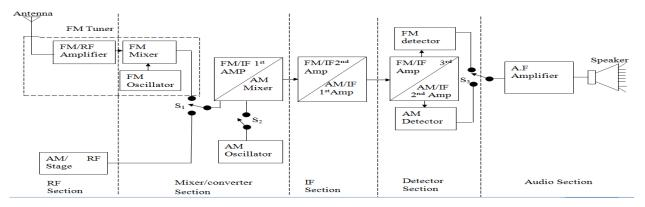
Figure 1: the complete FM/AM Receiver
