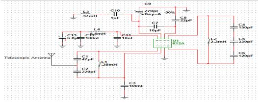
Fig 5: AM Double- balanced Mixer and Oscillator
