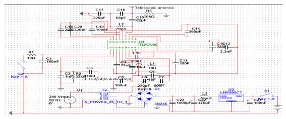
Figure 8 Designed complete FM Receiver
