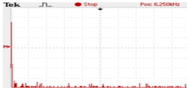
Fig. 16 Harmonics wave after selective harmonics elimination
