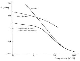
Fig. 4 : Graph of Penetration depth vs Frequency
