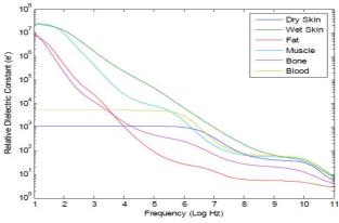
Fig. 3: graph of Dielectric Constant vs frequency (log, Hz)
