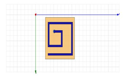
Fig. 5 : Design antenna at 4.73 GHz
