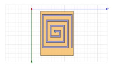
Fig. 8: Design antenna at 2.63 GHz
