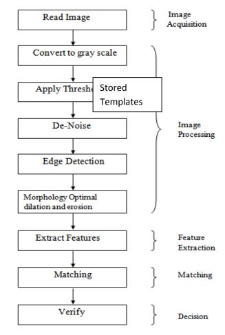
Figure 3(a): Hand Geometry Biometric System Module
