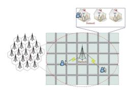
Figure 2.1: Femtocell Architecture
