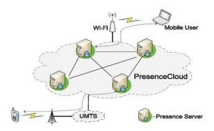
Fig 1. Architecture for presence cloud
