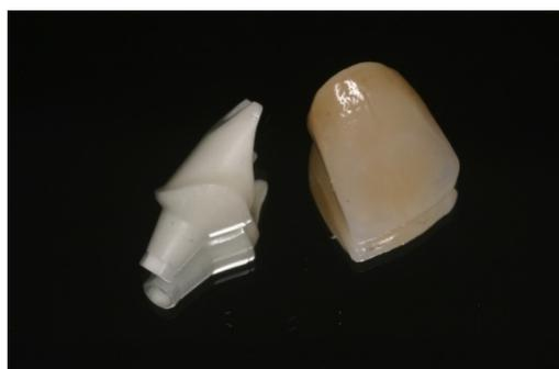
Figure 6. Zirconia atlantis abutment and crown.
