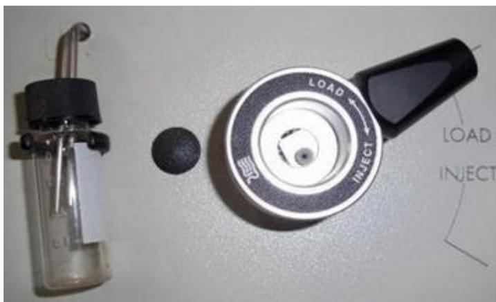
Figure 10. Inject (move the sample loop into the mobile phase flow).
