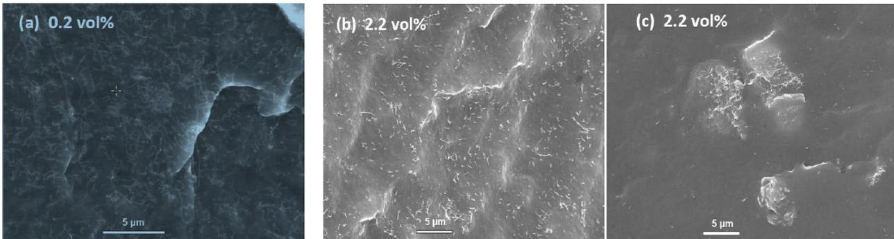
Fig.3. Uniform dispersion of functionalized SWNTs in the RET polymer is indicated, through Scanning Electron Microscope (SEM) micrographs, at both (a) 0.2 volume % and (b) 2.2 volume % filling fractions of the SWNTs. On the other hand, (c) non-functionalized SWNTs dispersed into the RET matrix exhibit clumping.(Prabhakar R. Bandaru .et.al.,Ref [60] cited in the below list)
