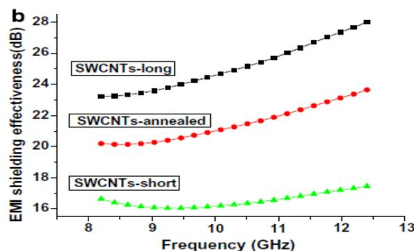
Fig. 4. EMI shielding effectiveness (SE) for SWCNT–epoxy composites. SE of SWCNT (15 wt %)–epoxy composites in the range of 8.2–12.4 GHz. ( Yongsheng Chen et.al .,Ref [62] cited in the below list)
