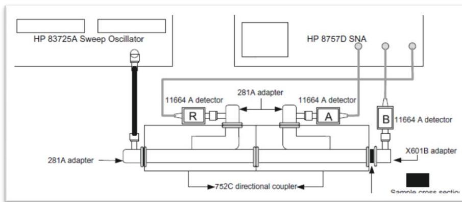
Figure2: Schematic sketch shows the instrument used to evaluate the EMI SE of the composites. ( Mohammed H.Al-S.et.al.,Ref [54] cited in the below list)
