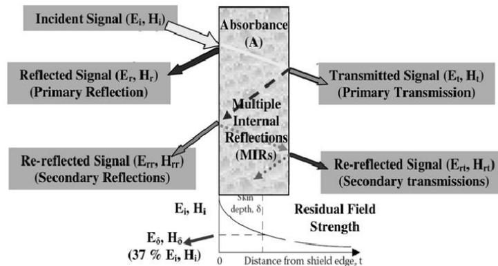
Figure 1. Graphical representation of EMI shielding. (Choudhary.V.et.al., Ref [8] cited in the below list
