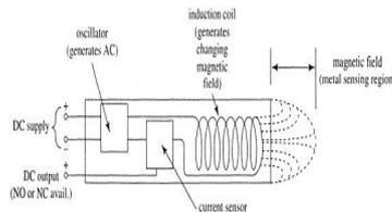
Figure4: Inductive Sensor Schematic
