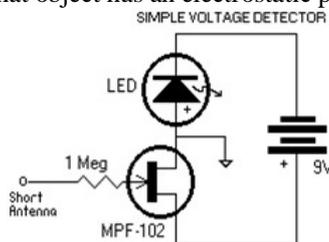
Figure3: The Discharge Sensor Schematic
