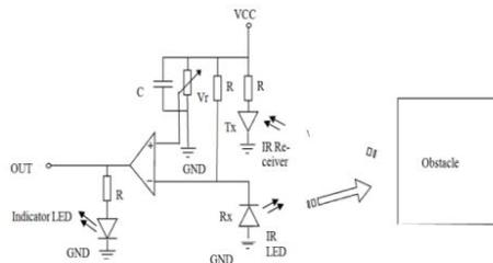
Figure1: The IR Sensor Schematic
