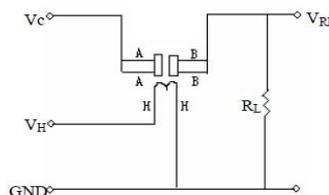
Figure2: This is the basic Circuit of GAS Sensor
