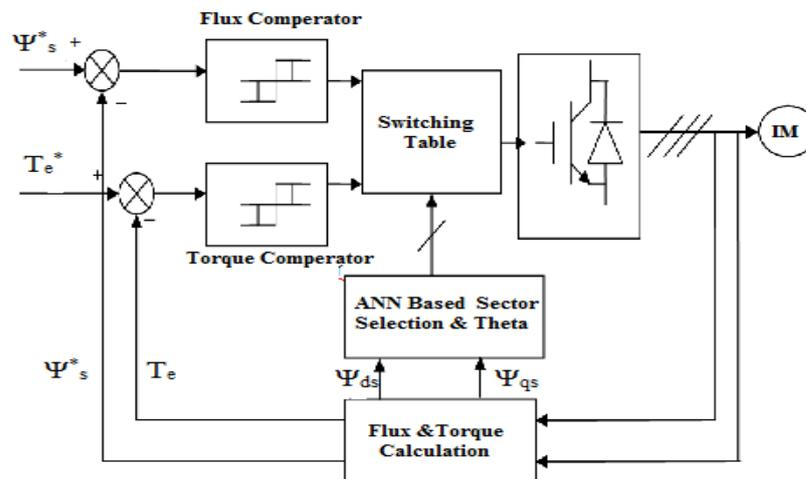
Fig. 2 Proposed ANN based DTC scheme
