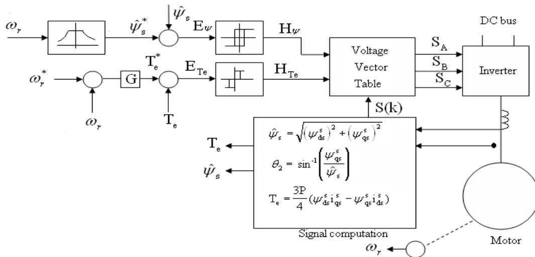
Fig.6 Direct Torque and Flux Control Block Diagram
