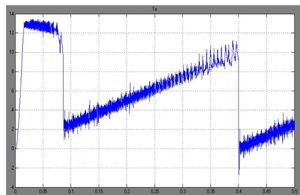
Fig.17 Electromagnetic Torque Response Waveform with ANN DTC
