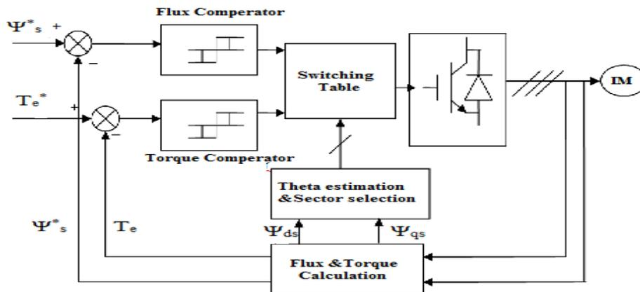
Fig. 1 Basic Direct Torque Control Scheme for AC Motor Drives
