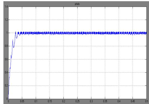
Fig.15 Stator Flux Magnitude of ANN Based DTC
