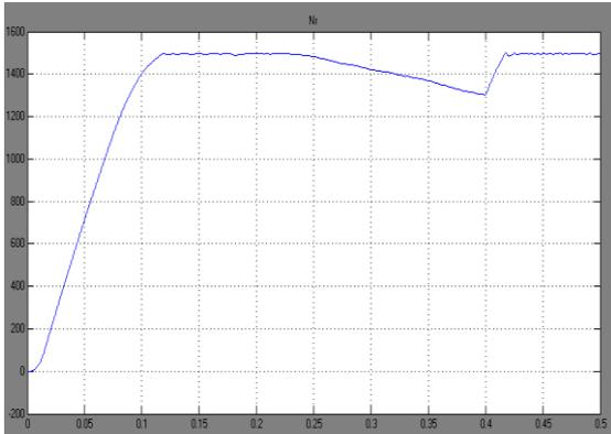
Fig.12 Speed of the Induction Motor using DTC with PID Controller
