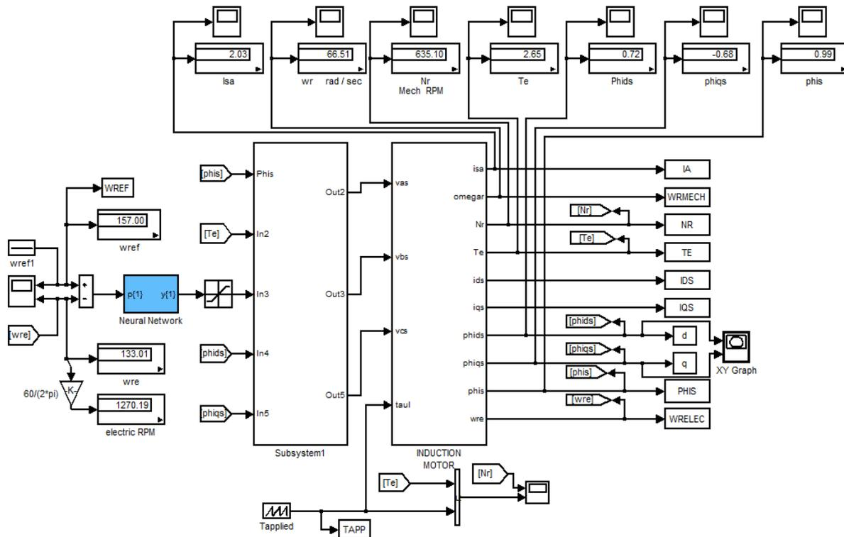
Fig.9 Simulation Block For DTC With ANN System
