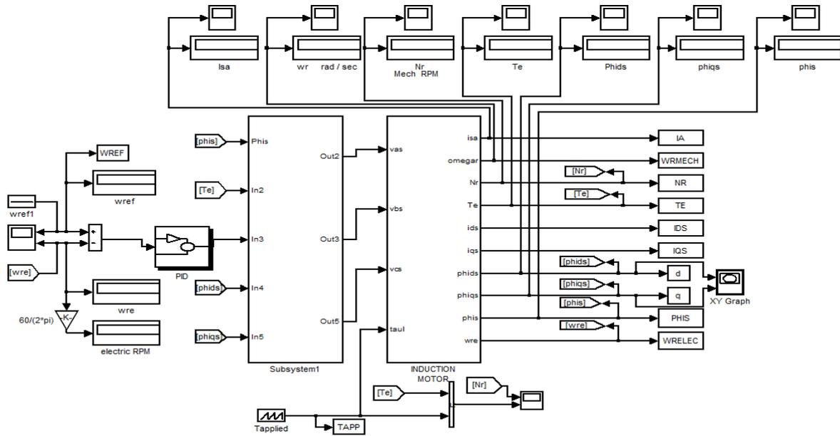
Fig.8 Simulation Block For DTC With PID System
