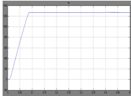
Fig.13 Speed of the Induction Motor With ANN Based SVM
