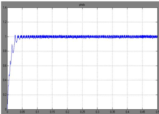
Fig.14 Stator Flux Magnitude conventional DTC
