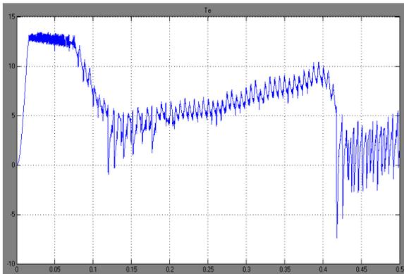
Fig.16 Electromagnetic Torque Response Waveform with PID
