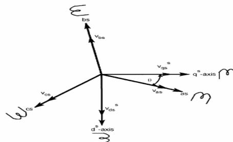
Fig.3 Stationary Frame a-b-c to d<sup>s</sup>-q<sup>s</sup> Axes Transformation
