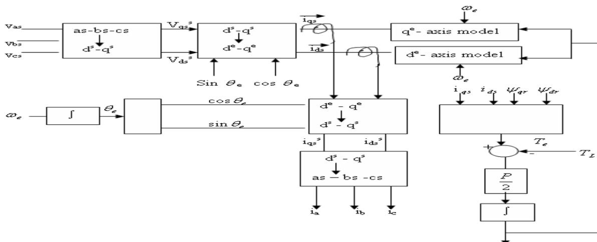
Fig.4 Synchronously Rotating Frame Machine Models with Input Voltage and Output Current Transformations
