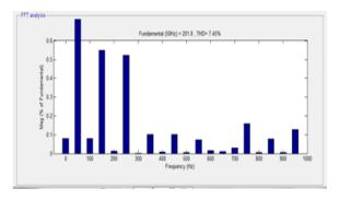
Fig 12 (d): FFT analyse of Fifteen-level inverter
