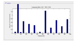
Fig 12 (c): FFT analyse of nine-level inverter
