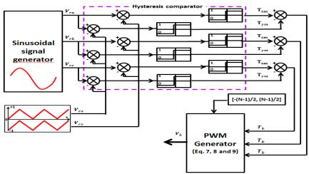
Fig. 5: Principle SPWM multilevel inverter control
