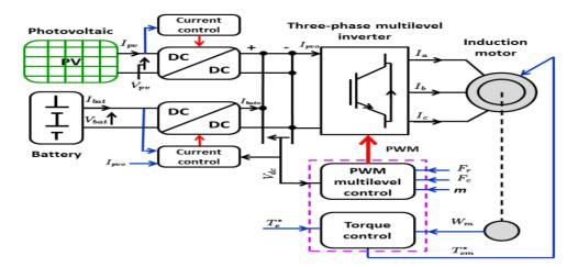
Fig. 1: Induction motor driven by PV-batteries standalone system using a controlled multilevel inverter
