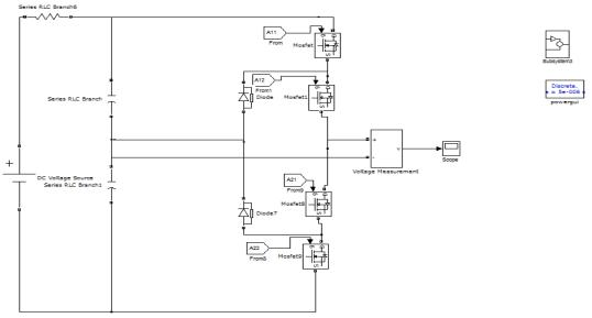
Fig (11) : Simulation diagram for a 3 level Multilevel inverter
