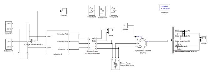
Fig: (10) MATLAB implementation of the Multilevel inverter fed an induction Motor
