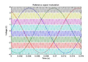
Fig. 7: Modulation signals of nine-level SPWM
