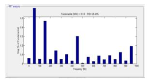
Fig 12 (b): FFT analyse of Five-level inverter
