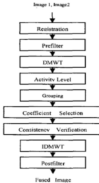
Fig. 4 Image fusion algorithm based on 2D-DMWT[3]
