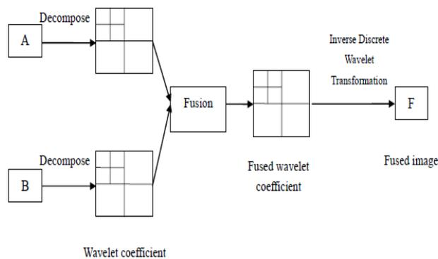
**Fig 2. Wavelet Based image fusion**
