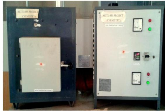
Fig.2: Diagram shows the high temperature furnace. As the paste which is applied over the material is in wet condition, it has to be dried off before it is taken for Induction boriding.
