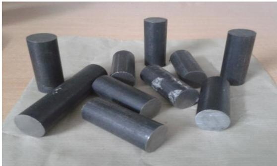
Fig. 1: high speed steel of M2 grade.
