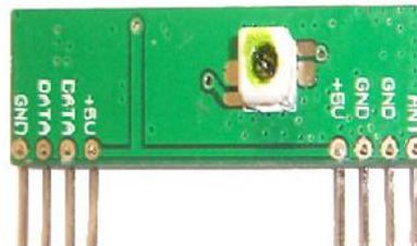
Fig. 4. RF Receiver STT-433MHZ.
