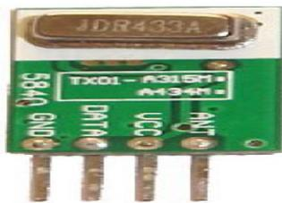
Fig. 3. RF Transmitter STT-433MHZ
