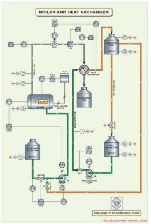
Fig. 1: Boiler and Heat Exchanger
