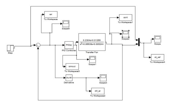
Fig. 4: Simulation for Boiler and Heat Exchanger Temperature Loop
